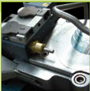
New cooling welding time indicator
